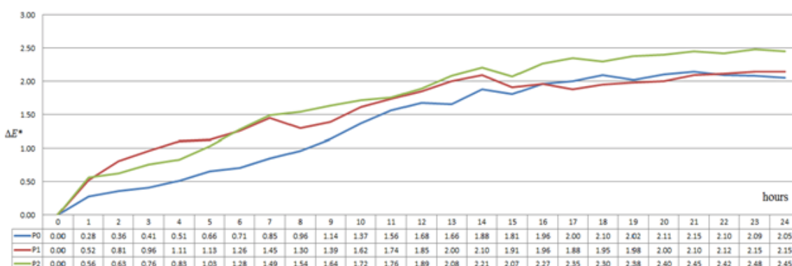
Fig. 5. Evolution graph of the \Delta E^* index on calcareous-rock surfaces exposed to UV radiation
